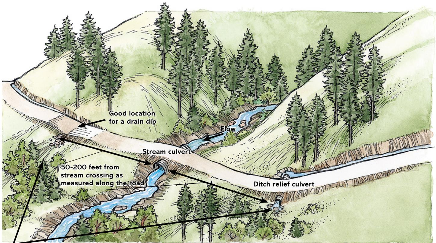
Ditch drainage should be directed into vegetation and undisturbed soil filter, and not allowed to continue flowing down the ditch and into the stream.
