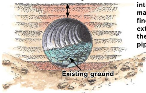
Tamp backfill material at regular intervals. Base and sidewall fill material should be compacted from finer soil particles. Fill height should extend at least 18 to 24 inches above the top of the culvert to protect the pipe from damage by traffic.
