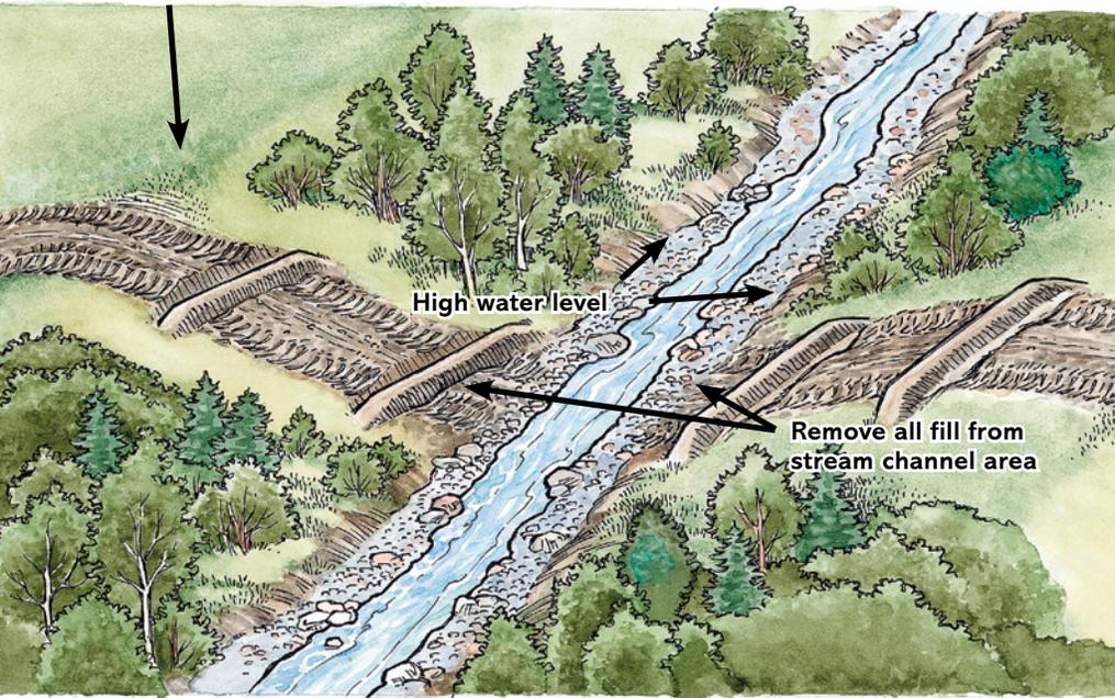
Construct water bars to divert runoff from temporary stream-crossing approaches. Construct them as soon as crossing use has ended and before the rainy season.
