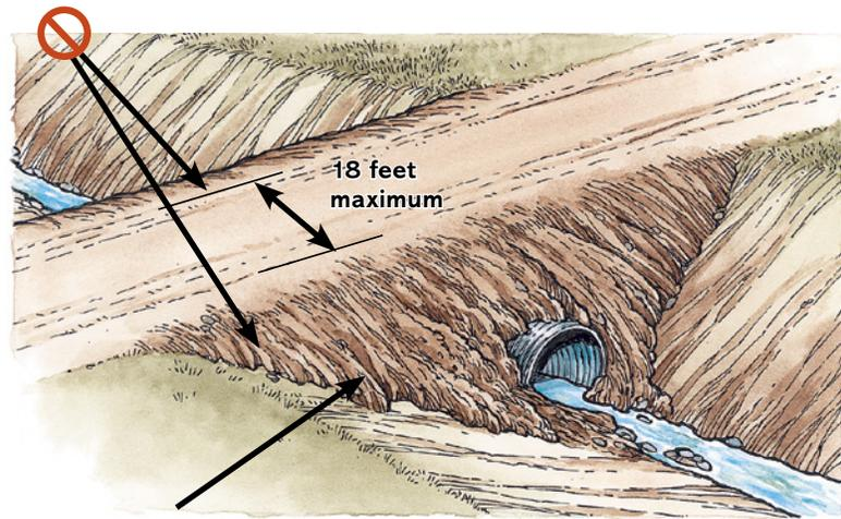
**Culvert outlets that are too narrow and set too high cause water to undercut the road fill and streambed.**
