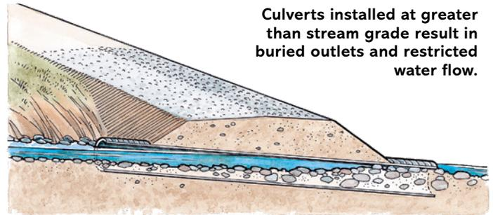
**Never use a stream crossing to dispose of excess material. The wider road surface increases risk of this material entering the stream.**
