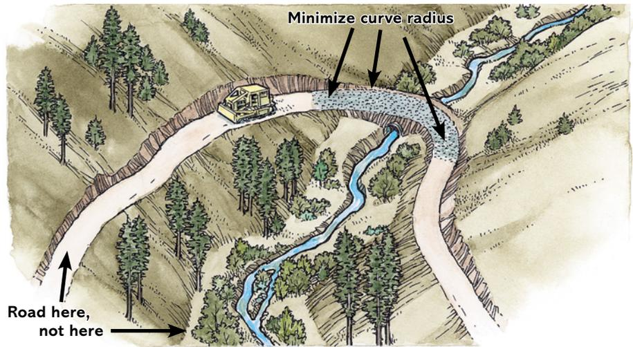
**Locate the road on side slopes of up to 50% grade when possible, rather than near the channel.**
