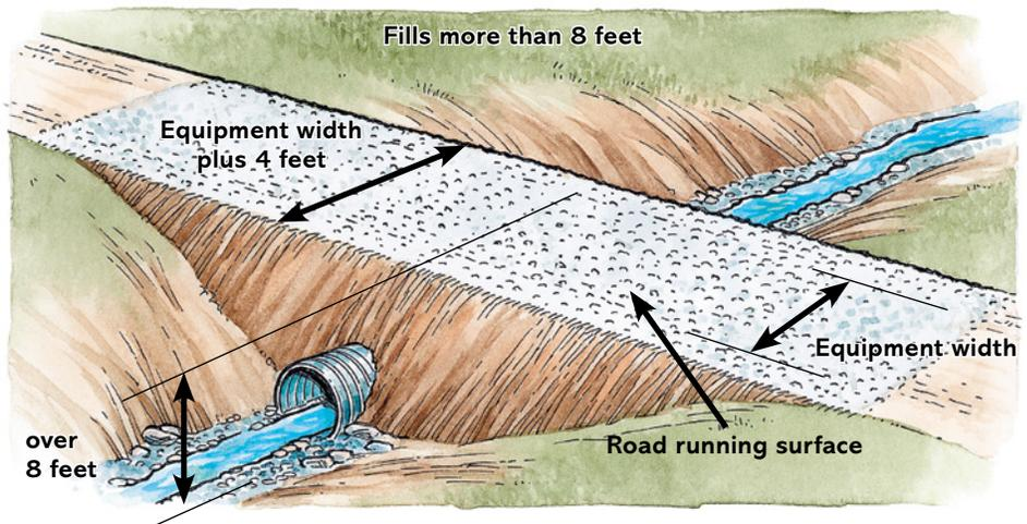
**Fill depth is measured from the road running surface to the stream bottom at the downstream side. Fills more than 8 feet deep must be designed in accordance with road construction and stream crossing fill rules, except that temporary crossings are not required to withstand a 100-year flood.**
