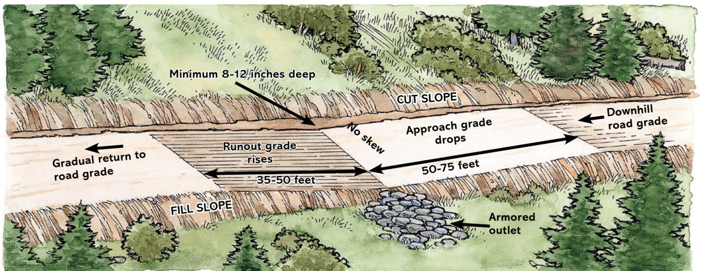
This drain dip bottom is sloped to carry water from the inside to the outside of the road surface and onto natural ground.
