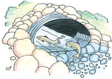
Water may be too shallow for fish to swim. Bare pipes frequently result in shallow water, leaving fish only partially submerged and unable to get maximum thrust from tail and body movements.
