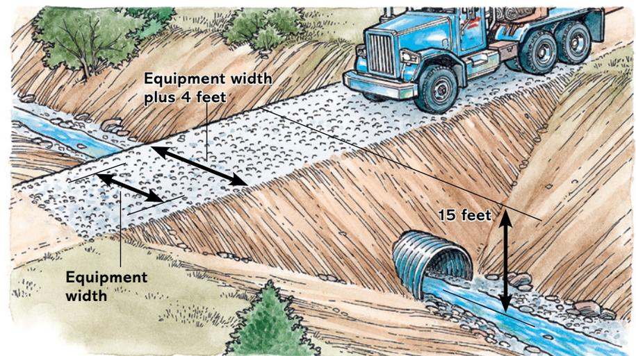
**Measure the fill depth from the road-running surface to the stream bottom at the downstream side.**
