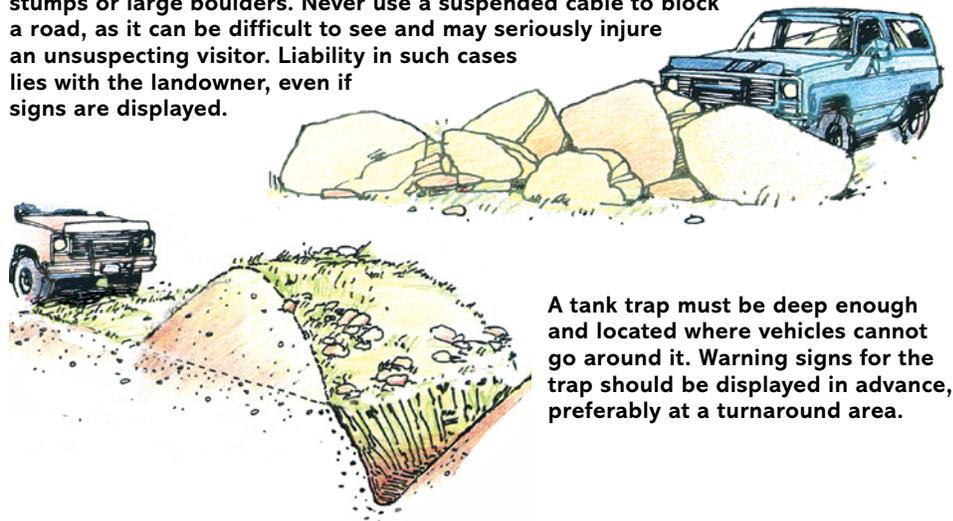
**A tank trap must be deep enough and located where vehicles cannot go around it. Warning signs for the trap should be displayed in advance, preferably at a turnaround area.**
