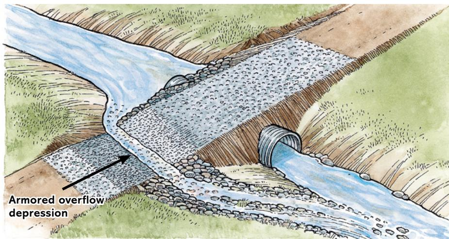
**This vented ford is a cross between a ford and a culvert crossing. Water passes through the culvert during normal flows, but the structure can accommodate peak stream flows across a ford section during large storms. Any permanent culvert in a stream needs to be sized for the 100-year peak flow.**
