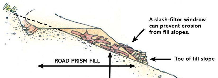
**Always avoid mixing stumps and other vegetative debris into the road fill. Over time, it can lead to road slumping and failure.**
