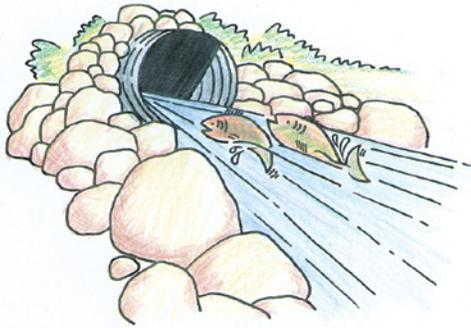
Fish may not be able to swim fast enough to overcome culvert water velocity that develops in culverts narrower than the width of the stream. Rule of thumb: Water moving through a bare culvert that is turbulent (uneven water surface or whitewater) is probably a fish-passage barrier.
