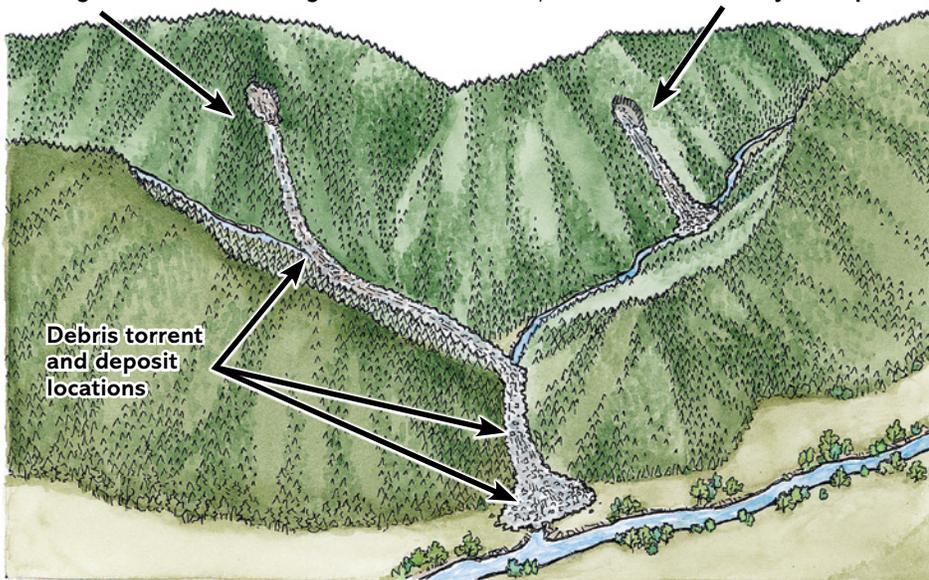
This illustration shows the action of two landslides. Landowners who conduct operations on slopes need to evaluate the potential for landslides. Many locations prone to rapidly moving landslides don't show evidence of prior landslides.
