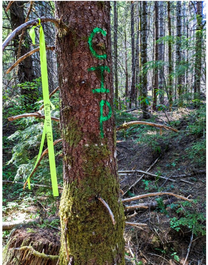
**Right:** The channel initiation point (CIP), visible in the lower right-hand corner of the the image and shown appropriately marked according to the survey protocols (permanent tree marking paint optional), is the most upstream location where a discernable channel with a stream bed and banks is observed, whether it contains flowing water or not.
